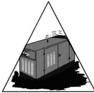
Ground too uneven or soft. Set incorrectly positioned
