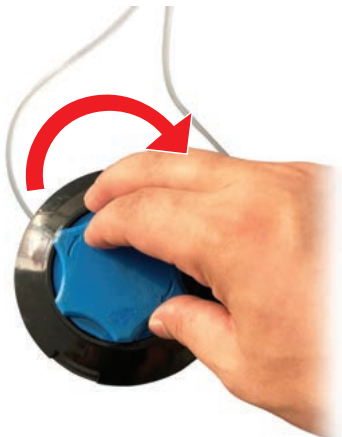
STEP 5 : Turn the blue centre piece clockwise until there is 20cm of line remaining.
