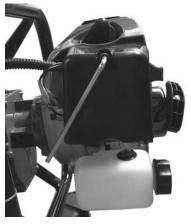
Loosen the screw on the air filter casing. Remove the air filter cover and check it.
