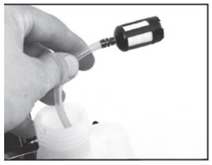
Pull old filter from fuel pipe and replace with new filter.
