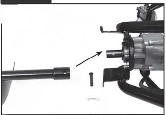
Place the motor casing on a work bench. Place the earth auger on the drive shaft, ensuring that both holes are aligned.
