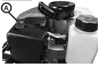
After running for 10 seconds or so, squeeze the throttle trigger to release the choke lever (A) to the RUN position.
