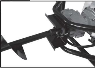
Insert the drive pin. Secure with R-pin.
