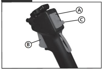
Put the stop switch (A) into the start position.
