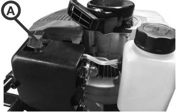
If the engine is cold, move the choke lever (A) to the START position. The choke lever opens and closes the choke in the carburettor.
