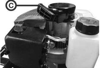
4Lightly pull on the starter cord (C) until you can feel resistance, then pull on the cord quickly and firmly until the engine starts.
