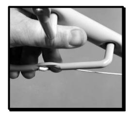
6. Check the cable lies flat and has not snagged on any other part of the mower.
