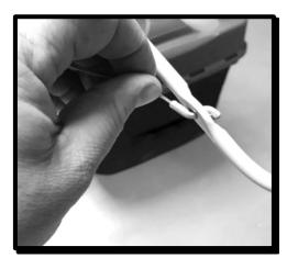
5. Refit the lever back into its location hole on the main handlebar.
