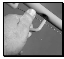
3. Insert the end of the cable in to the location hole on the lever
