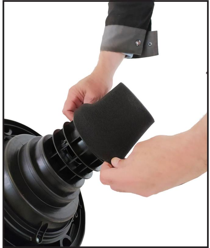
**⚠ NOTE :** Before using to vacuum for wet cleaning, remove all dirt and debris from the tank. The foam intake filter must be used to vacuum up wet debris. Unplug the power cord from the wall outlet before removing the motor assembly from the tank.
