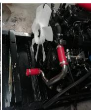
10. With the radiator removed, you can access the back of the fuel pump. Remove the cover to reveal the timing gears.
