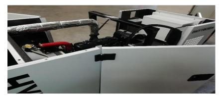
5. Remove the breather pipe which witch is attached from the engine to the canopy. It is located just above the starter motor.
