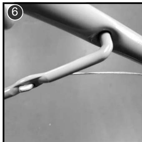
Check the cable lies flat and has not snagged on any other part of the lawnmower.
