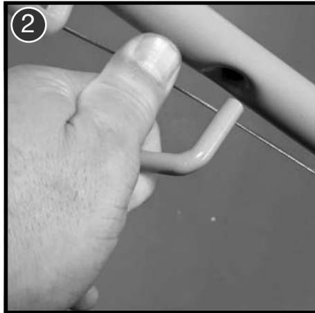
Gently prise the lever inwards from its locating hole in the main handlebar.
