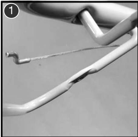
Follow the cable you want to attach and determine which lever it will attach to.
