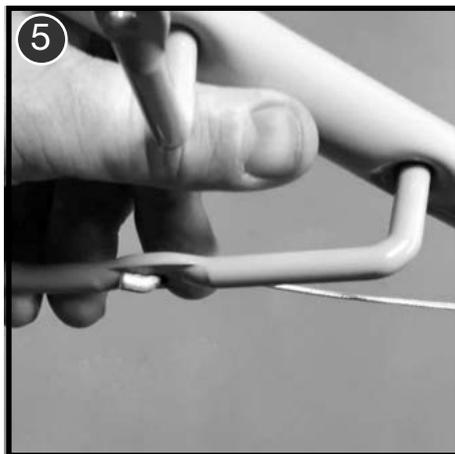
Refit the lever back into its location hole on the main handlebar.
