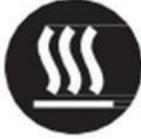
3.3.13. **WARNING** Exhaust heat/gases can ignite combustibles, structures or damage fuel tank causing a fire.
