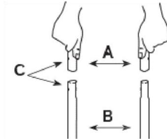
5.5. **NOTE** It may be necessary to move the handle supports from side to side in order to align the handle so it will slide over the handle supports.
