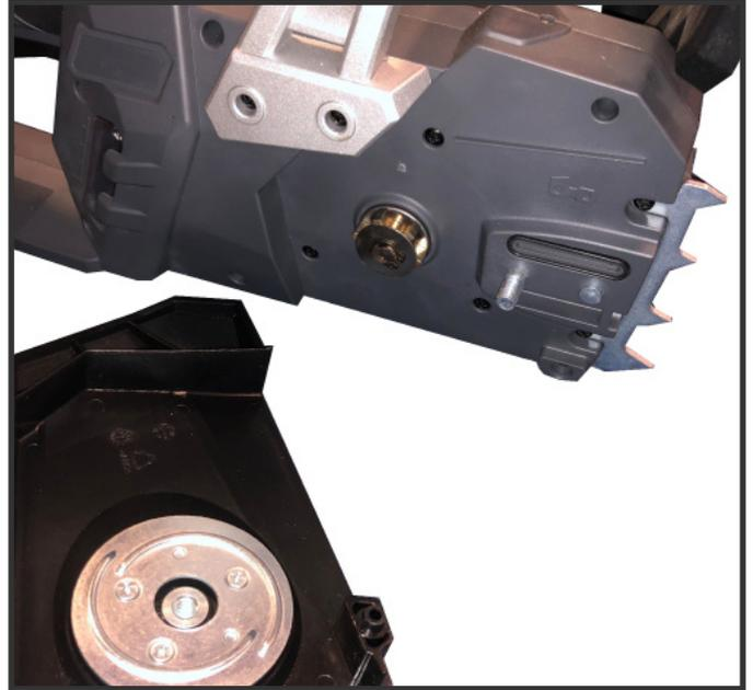
3. Place the chain onto the bar. The chain bar is marked with an arrow that shows you the direction in which the chain will travel. Make sure all the chain links are seated correctly into the groove in the chain bar. The cutting teeth on the upper side of the bar must point forward, as marked on the bar.
