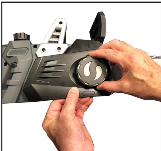
2. When the chain needs re-tensioning, loosen the large adjuster knob two to three turns until the tension on the bar is released, then tighten clockwise until tension is applied to the bar, then a further one and a half turns.
