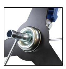
2.43 To remove the brush cutter blade, reverse the procedure.
