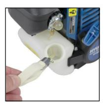
7.22 Reinstall the fuel filler cap and tighten securely.
